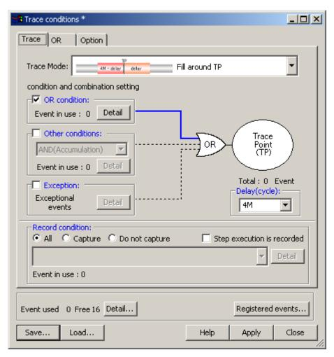
Figure 3.34 Trace conditions dialog box (Fill around TP)
